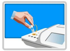
**8.** Place the cuvette in one of the incubation cells and start the timer by pressing the timer icon.
