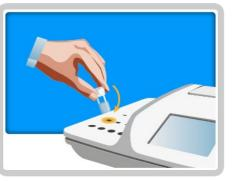
**14.** Place the cuvette in one of the incubation cells and start the timer by pressing the timer icon.
