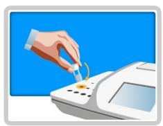
**15.** Place the cuvette in one of the incubation cells and start the timer by pressing the timer icon.
