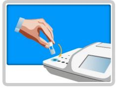
**17.** Place the cuvette in the cell marked with the blue light and press READ to perform the photometric reading.
