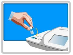
**10.** Select the cuvette to be read from the display. Place the cuvette in the cell marked with the blue light and press READ.
