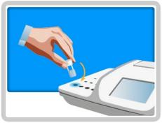
**16.** Place the cuvette in the cell marked with the blue light and press READ to perform the photometric reading.
