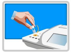
**9.** Place the cuvette in one of the incubation cells and start the timer by pressing the timer icon.
