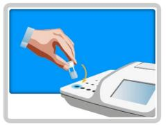
**11.** Select the cuvette to be read from the display. Place the cuvette in the cell marked with the blue light and press READ.
