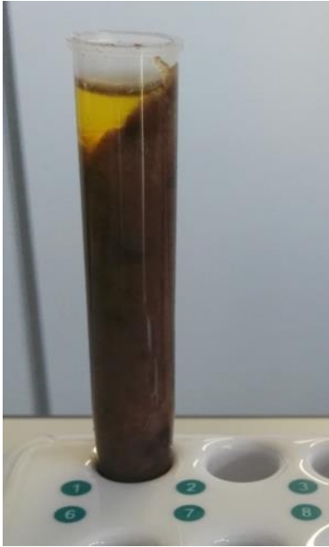
Figure 1. Fatty substance extraction with the CDR FoodLab® system
