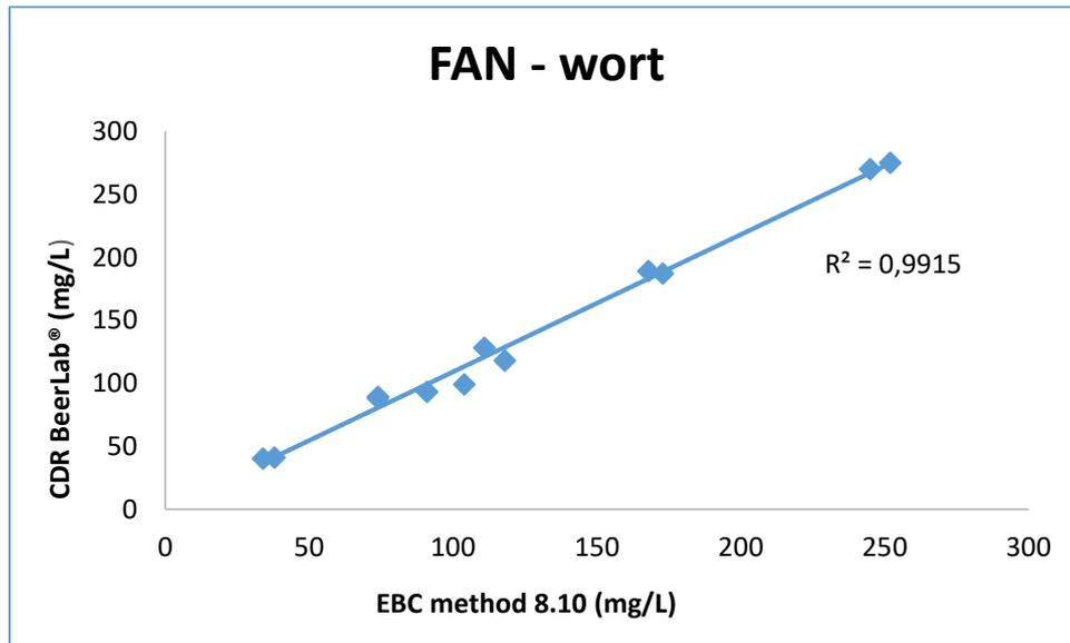
Figure 4 Correlation between FAN content in worts measured with CDR BeerLab® and EBC method 8.10.
