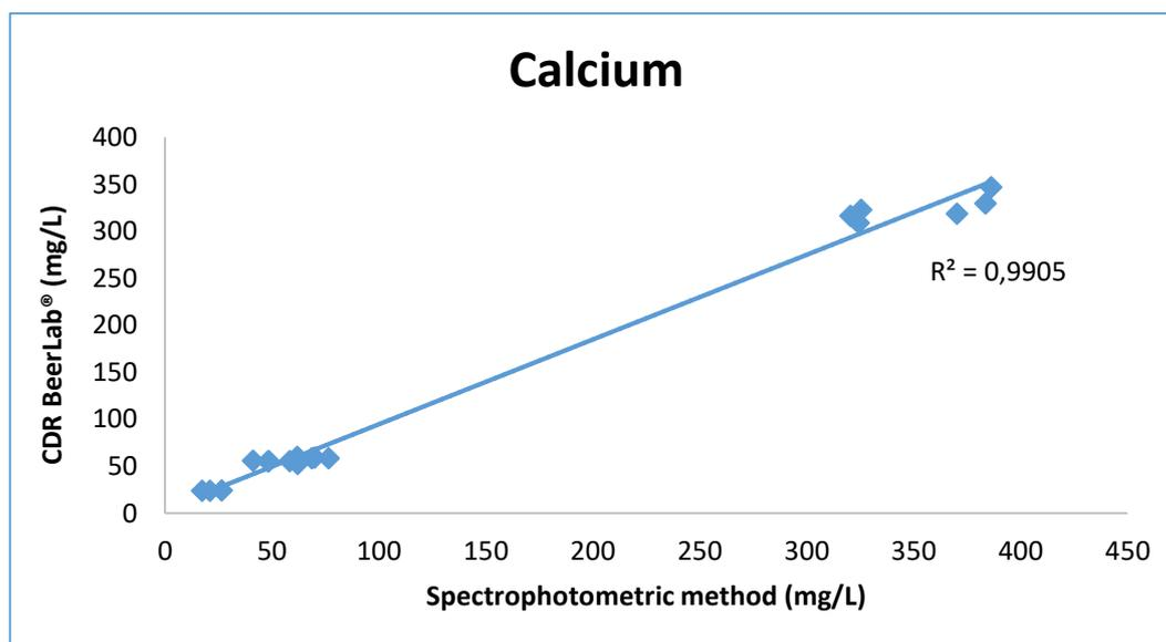
**Figure 10 Correlation between calcium content in waters with CDR BeerLab® and spectrophotometric method.**
