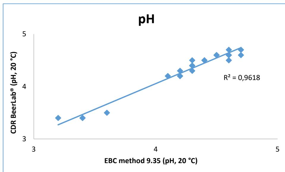
**Figure 2 Correlation between pH values measured at 20 °C with CDR BeerLab® and EBC method 9.35.**
