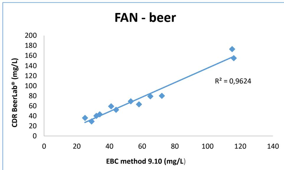
Figure 5 Correlation between FAN content in worts measured with CDR BeerLab® and EBC method 9.10.
