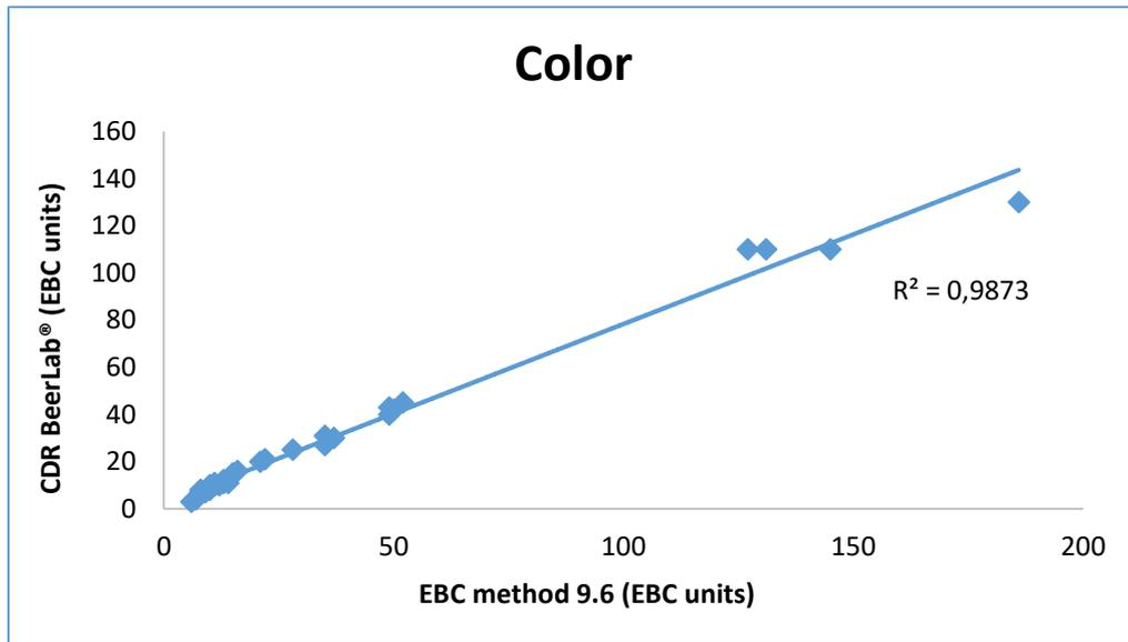
Figure 3 Correlation between color units measured with CDR BeerLab® and EBC method 9.6.
