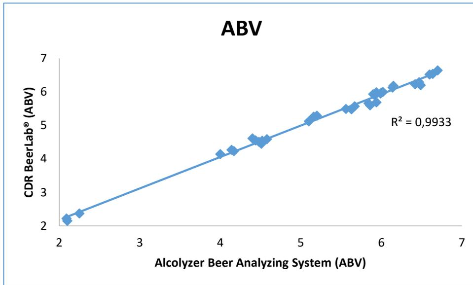
**Figure 1 Correlation between ABV values measured with CDR BeerLab® and Alcolyzer Beer Analyzing System.**
