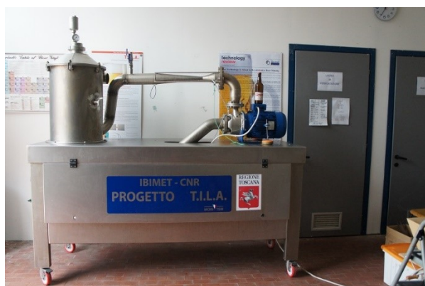
Picture 1. Pilot plant brewing by hydrodynamic cavitation
